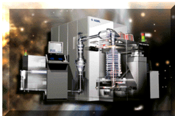
130 nm volume production lithography system. ASML PAS5500/750E
